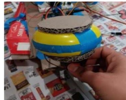
Figure 3: Inflatable wheel. The image shows the prototype flexible wheel I used during my preliminary experiment.
